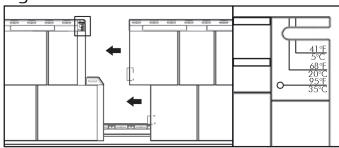
5-Begin the second row by cutting the first panel with 16"(40,64cm) increment from the cutting line of the first row. Hooking the lower panel section with the top hooks of the last installed row. To eliminate stacking seams, alternate the cut positions for the following rows. (Figure E)
